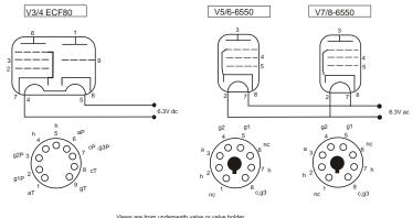
Views are from underneath valve or valve holder h = heater hct = heater centre tap c = cathode a = anode g1= grid 1 g2 = grid 2 g3 = grid 3 nc = no connection (T=triode P=pentode for V1)
