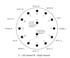
FRONT VIEW (SHOWS ORIENTATION OF SELECTOR SWITCH CONTROL WASHER TO 6/2 POLE POSITION)
